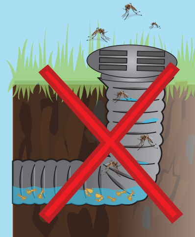
Un-screened yard drain
