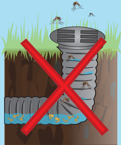
Un-screened yard drain
