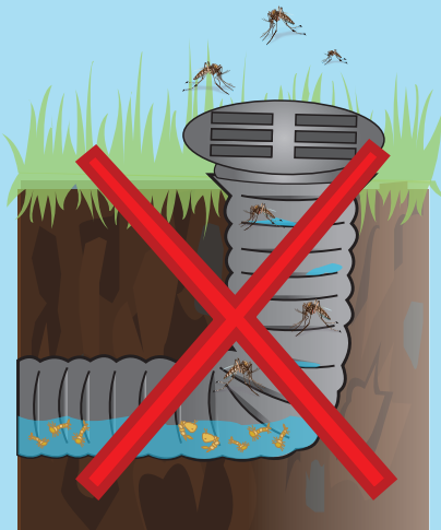
Un-screened yard drain
