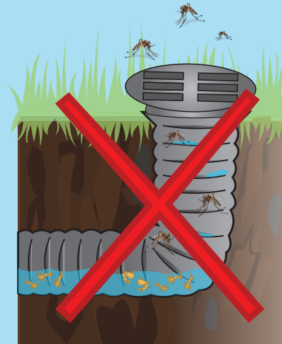
Un-screened yard drain
